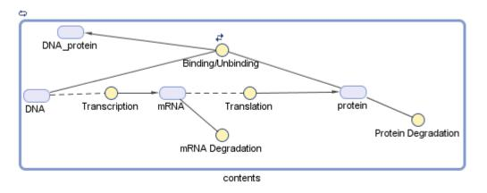
Notice the use of dashed lines for species that are both reactants and products in a reaction (modifiers). Note the indicator for a reversible reaction associated with the Binding/Unbinding reaction.
